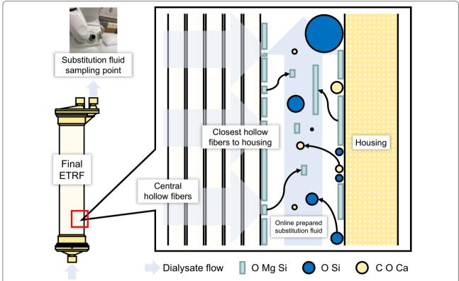
**Fig. 4** Schematic diagram of insoluble particulate matters adhering to the final ETRF. Schematic diagram of insoluble particulate matters adhering to the final ETRF and discharging to online prepared substitution fluid. In constituent elements, C is carbon, O is oxygen, Mg is magnesium, Si is silicon, and Ca is calcium. ETRF stands for endotoxin-retentive filters
