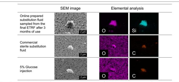
**Fig. 1** SEM image and EDS mapping of particles in online prepared substitution fluid. SEM image and EDS mapping of particles in online prepared substitution fluid sampled from the final ETRF after 3 months of use, commercial sterile substitution fluid, and 5% glucose injection. In EDS mapping (elemental analysis), brown is C, pink is O, and turquois blue is Si. SEM, scanning electron microscopy; EDS, energy-dispersive X-ray spectrometry; ETRF, endotoxin-retentive filters
