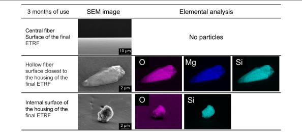
**Fig. 2** SEM image and EDS mapping in the final ETRF. SEM image and EDS mapping of the central fiber surface, hollow fiber surface closest to the housing, and internal surface of the housing for the final ETRF with 3 months of use. In EDS mapping (elemental analysis), brown is C, pink is O, blue is Mg, turquois blue is Si. SEM, scanning electron microscopy; EDS, energy-dispersive X-ray spectrometry; ETRF, endotoxin-retentive filters
