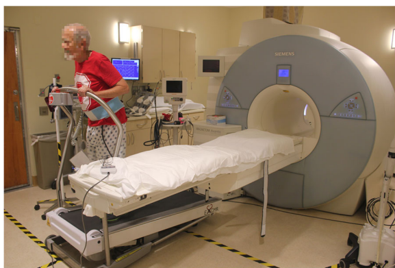
Fig. 1 Cardiovascular magnetic resonance (CMR) compatible scanner adjacent treadmill, developed and utilised in ischaemia studies by the Ohio State University Research group [27], reduces transfer times for post stress CMR imaging, whilst still allowing a diagnostic 12-lead ECG treadmill test and a simultaneous maximal oxygen uptake test, if required
