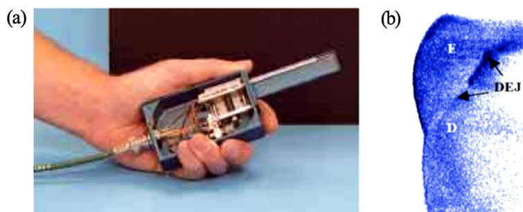
Fig. 3 a The first OCT handpiece and b the image for visualization of enamel (E), dentine (D), and dentine–enamel junction (DEJ) by Colston et al. (Adopted with permission from [78])
